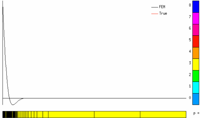
Figure 11: Bending moment M = M(x) in the shell problem at t = 1/1000 . DPG method with optimal test functions corresponding to an automatically generated h -mesh with 884 D.O.F. (black) overlaps the true solution (red).
