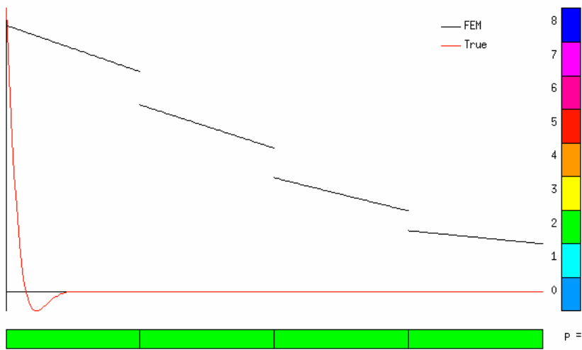
Figure 7: Bending moment M = M(x) in the shell problem at t = 1/1000 . Initial mesh with standard test space norm.
