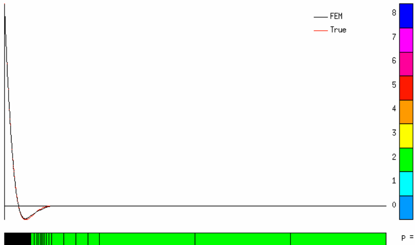
Figure 10: Bending moment M = M(x) in the shell problem at t = 1/1000 . DPG method with optimal test functions corresponding to an automatically generated h -mesh with 1360 D.O.F. (black) and the true solution (red).
